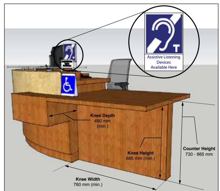
Figure 100: Dimensions of Accessible Service Counter
