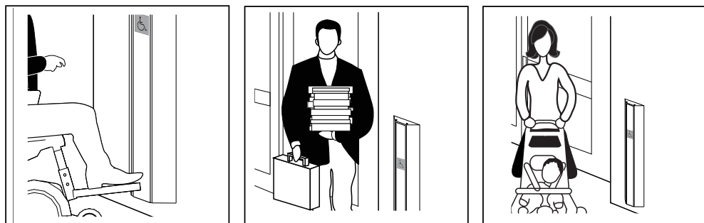
Figure 39: Example of Control for Power Door Operator Promoting Universal Use
